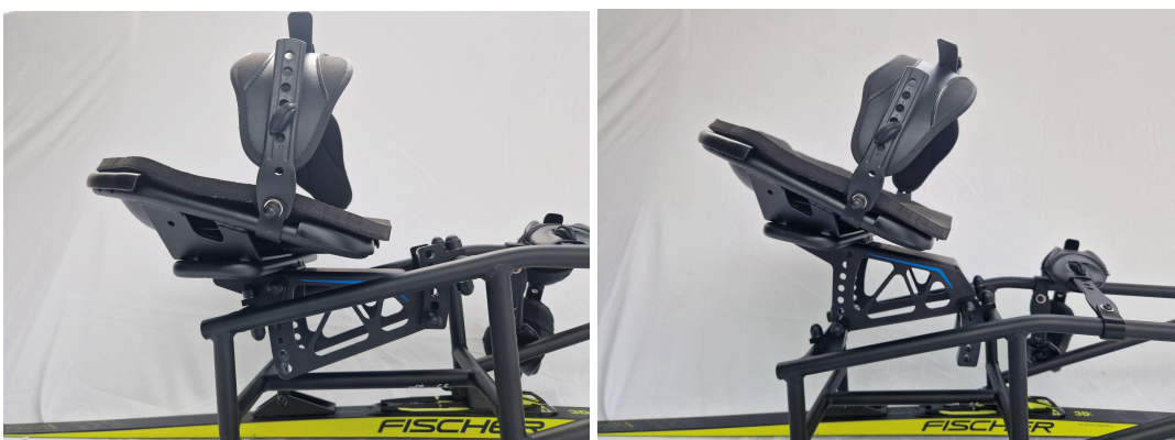
Figure 3.2.1d - Seat width and height adjustments (Torque = 5Nm).
