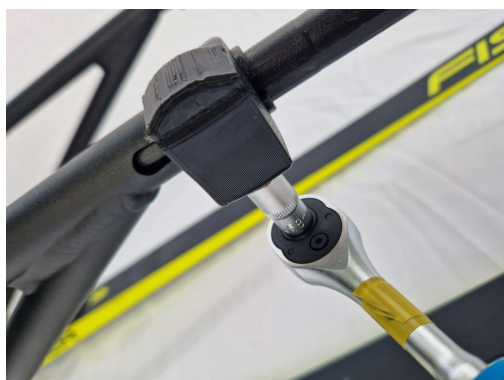
Figure 3.2.1c.1 Loosen/Tighten bolt on pipe clamp (Torque = 8Nm).
