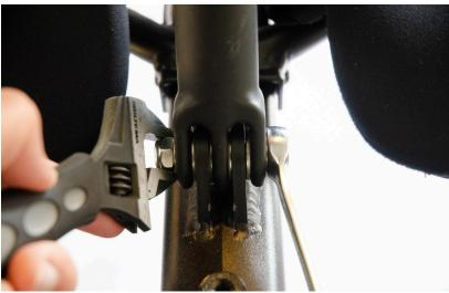
Figure 4.1.3 - Tightening seat arm (right) and seat post (left)
