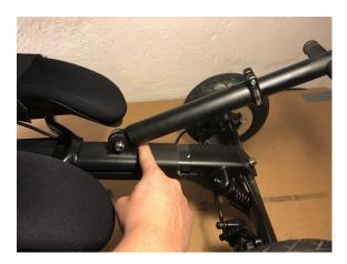
Figure 6.4.1 - Danger of trapping fingers during folding.
