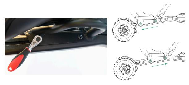
Figure 4.1.4 - Tightening front slider
