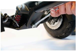
Figure 4.1.2 - Tightening steering system
