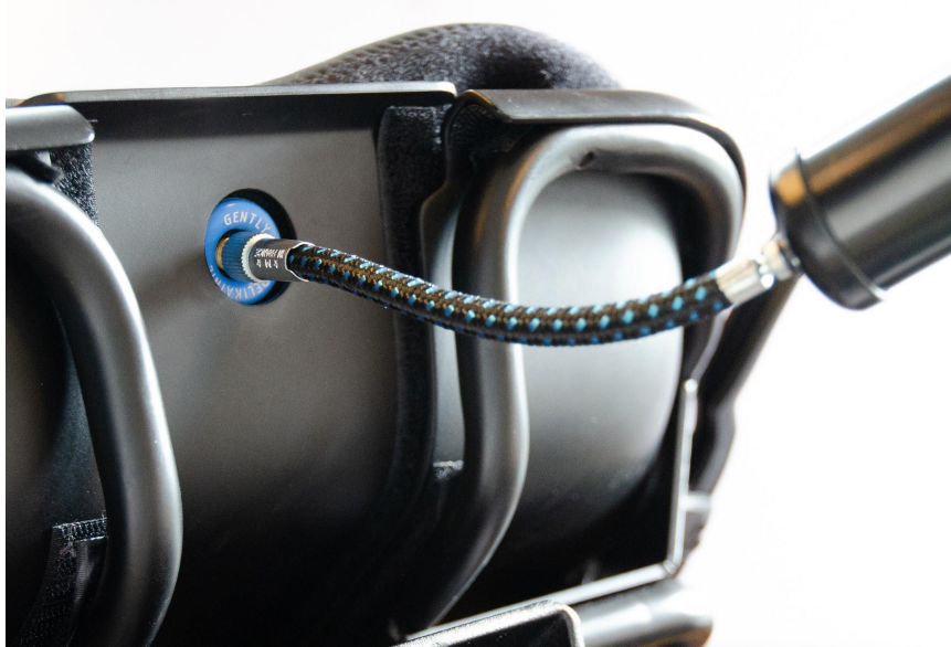
Figure 3.4.9 - Pump and adapter mounted for draining air.
